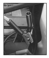
Now connect the black negative (-) cable to the negative (-) terminal of the good battery. Use a remote negative (-) terminal if the vehicle has one. Your vehicle's remote negative (-) terminal is marked GND.
